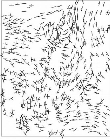
Figure 12.5 Orientation map of foliation strikes of the data shown in Figure 12.3. The strike tick marks represent the horizontal projection of the dip line using the \vdash symbol.
